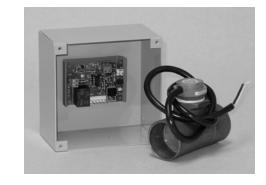
The *ISIMET* Emergency Shower Monitoring Unit is a companion component to the ISIMET Utility Controller System. The unit is provided with a micro-flow switch, time delay circuit, junction box, and mounting hardware. The unit is not provided with a power source and must derive 24-vac operating power from the companioned Utility Controller.
